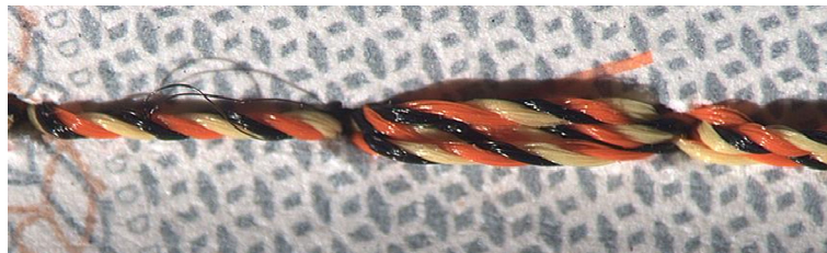
Figure 22: Example of genuine stitching thread (German passport).
