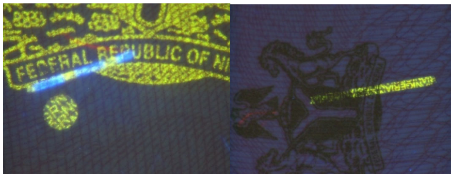
Figure 10: Example of a planchette (left) and a security fibre (right) with issuer branding visible under UV illumination (Nigerian passport)
