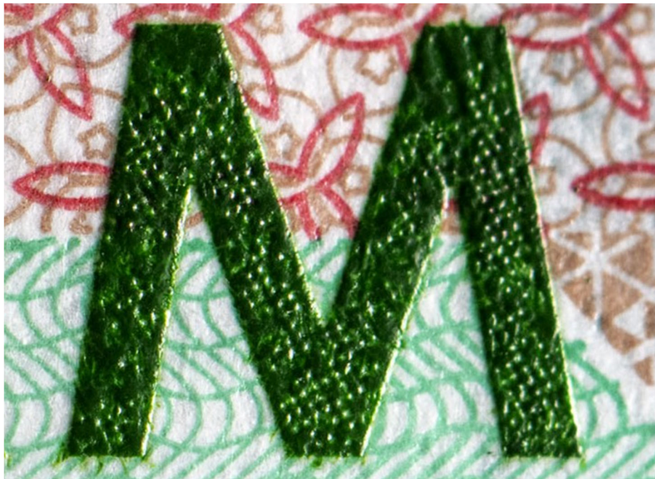
Figure 1: Example illustrating registration of multicolor offset printing and intaglio printing (Zambia 10 Kwacha Banknote — Credit: KEESING TECHNOLOGIES)
