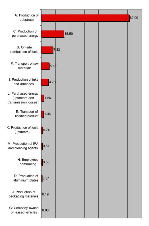
These values provide an illustrative example of proportions of  $CO_2$  emissions, and should therefore **not be interpreted** as representative values for the European printing industry in general. The company under investigation operates heatset printing facilities and produces magazines and advertising leaflets. It has in-house facilities for file content management, prepress, printing, finishing, and provides distribution services.
